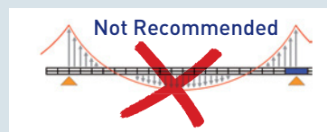
Never put the support under coupler.
